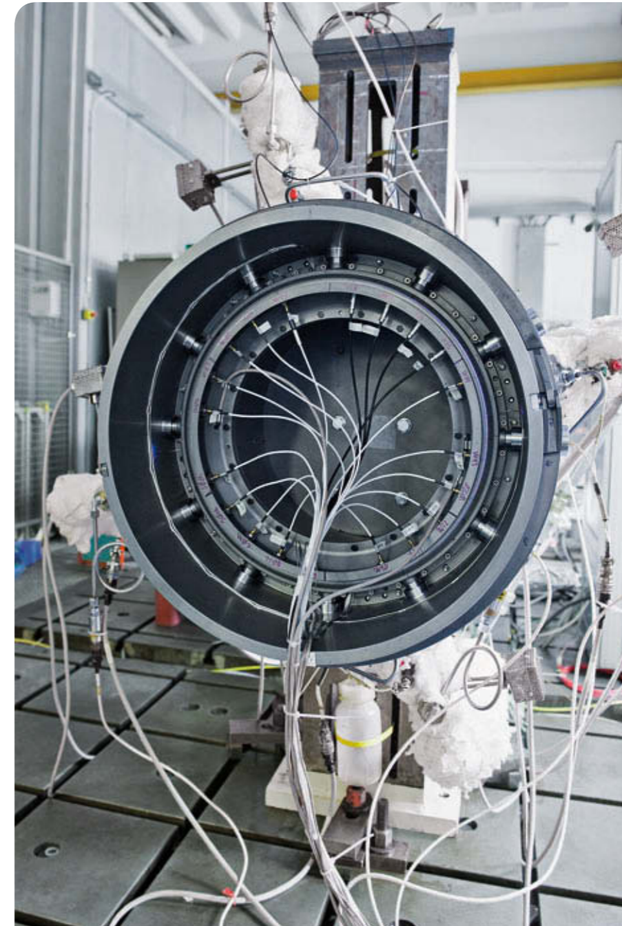
Setup for testing of the active clearance control system.
