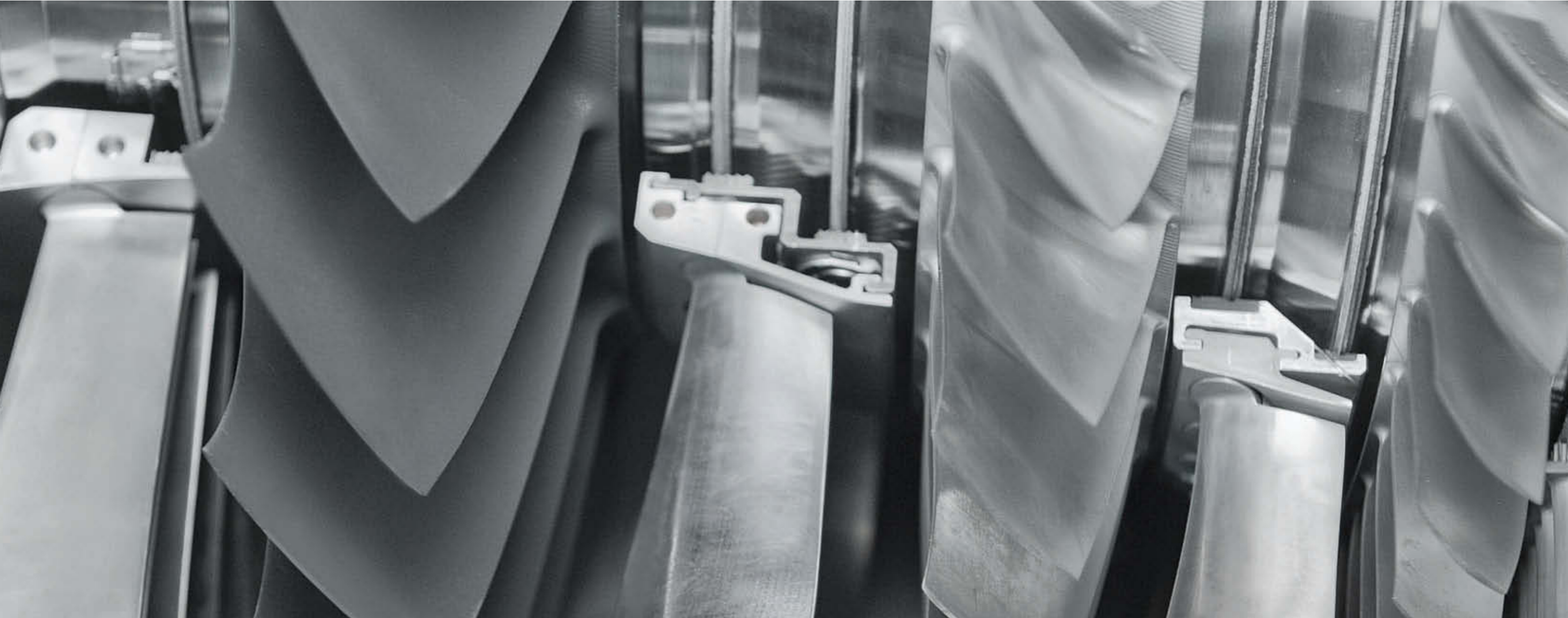
Active compressor on MTU's rig 260.
