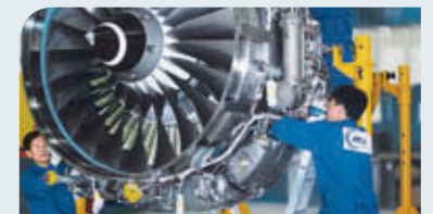
Assembly of a V2500 engine at MTU Maintenance Zhuhai.
