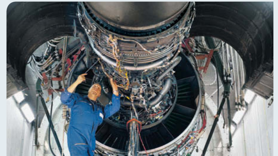
A Pratt & Whitney PW2000 in the development test cell of MTU.
