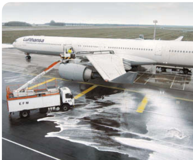
The glycol mixture is collected via drain channels in the tarmac.
