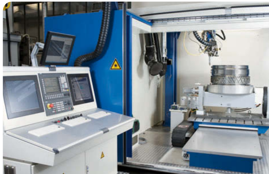
Adaptive laser powder cladding machine, a complex high-tech facility.
