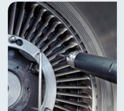
Adaptive milling of a low-pressure compressor stator.
