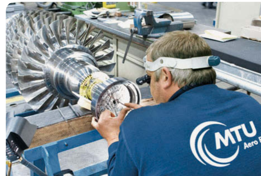
The new MAN hybrid axial compressor with the instrumentation being fitted.
