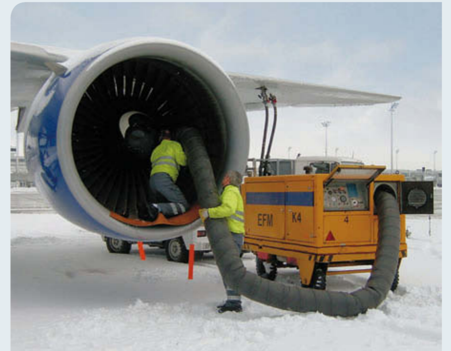
Ice in the engine intake is removed using hot air.
